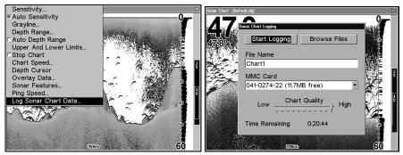
The Sonar Page menu with the Log Sonar Chart Data command selected (left). Sonar Chart Logging menu, with the Start Logging command selected (right). The MMC has 11.7 MB of free space, which will record the scrolling chart for 20 minutes and 44 seconds.
